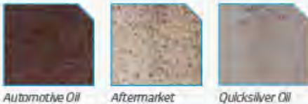
Photo shows NMMA FC-W Corrosion Test performance on Mercury cylinder strips.
